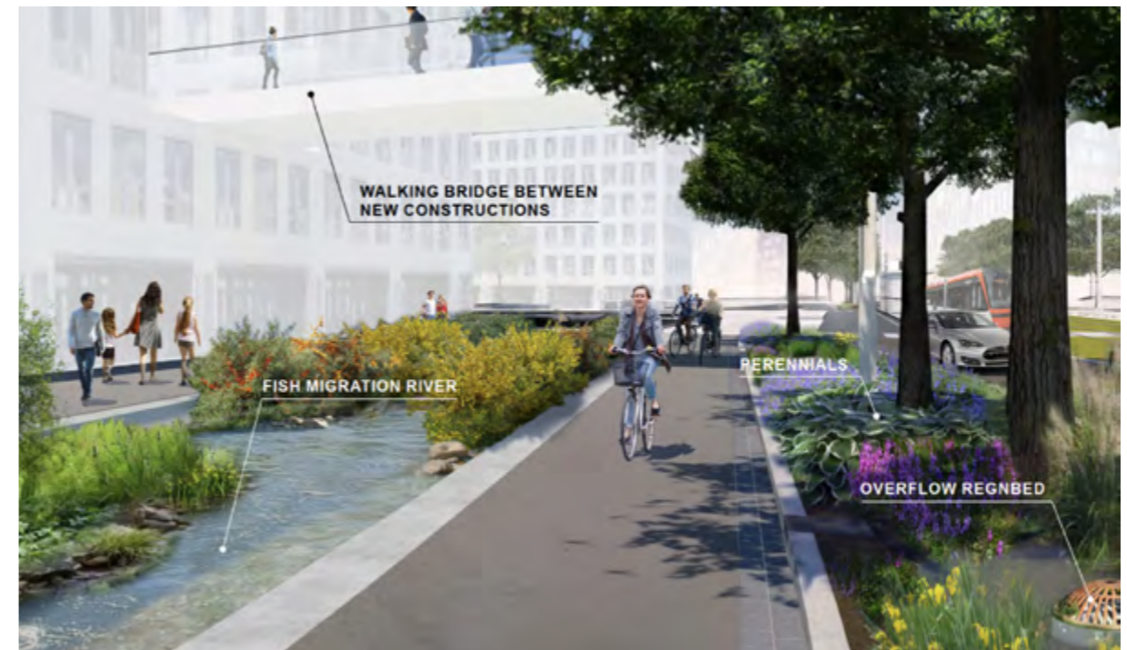
Bringing back the sea trout by the restoration of a historically important fish migration route. The fish migration river has been designed in close consultation with a fish biologist. The water speed, waterfalls, water depth and shade spots all determine the success of the route. In addition, the planting plan, including its trees and shrubs, is inspired by the natural vegetation near mountain streams. Location: Mindemyren in Bergen, Norway. Visualisation: Sweco in the Netherlands
